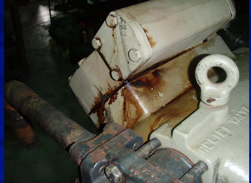
Occasionally you may find that the compressor oil drops while running, but returns relatively quickly during the off cycle. This is likely due to worn piston rings allowing 'blow by' of the discharge gases into the compressor sump. This pressurizes the sump above suction pressure, trapping the returning oil in the motor compartment. When the compressor shuts down, the pressures equalise and oil returns through the crank case oil check valve.
